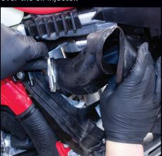
**14)** Reinstall shock top bolt. Confirm hose clamp is on intake boot. Reinstall intake boot by folding it in half vertically to aid getting it in airbox.
