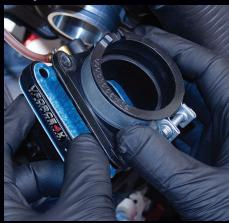
11) Place stock intake manifold on stock manifold plate. Install retaining bracket that protects oil injector ensuring it goes over the oil injector.
