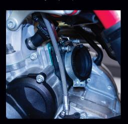
**5)** Using a ratchet with 8mm socket loosen and remove the reed valve screws.
