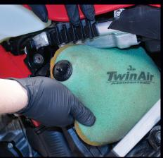
**16)** Reinstall air filter and side panel. Test throttle to confirm it fully returns prior to starting. Installation is now complete.
