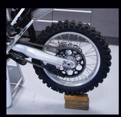
**3b)** We suggest using a wooden block to hold up the rear wheel to help keep the shock in place and out of the way.
