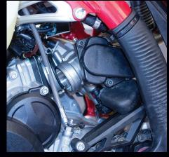
**4)** Loosen throttle body clamp then remove throttle body from intake manifold. You can zip tie it loosely to the subframe to keep it out of the way.
