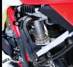
2) Begin removing intake boot. Remove the vent hose before completely removing intake boot. Leave hose clamp on intake boot to ease reinstallation.
