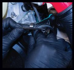
**6)** Remove intake manifold and place retaining bracket aside to be reused.
