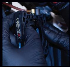
**9)** Take stock manifold plate with oil injector and place it into VFORCE4X with coring side facing you and oil line facing left. Push it into place.
