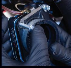
**12)** Install VFORCE4X using the supplied longer bolts ensuring retaining bracket tab is over oil injector. Tighten bolts to manufacture's torque specification.
