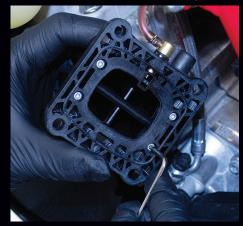
**7)** Use the supplied Torx wrench to remove screws on the back of stock reed cage, removing it from the manifold plate with oil injector. Do **not** remove oil line.
