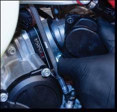
**13)** Install throttle body back in place aligning tab on throttle body to slot in intake manifold. Make sure vent hose is accessible. Tighten manifold hose clamp.
