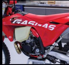
1) Remove side panel and air filter. Thoroughly clean all around airbox. Loosen hose clamp on intake boot.
