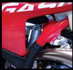
**3a)** On GASGAS and Husqvarna models remove the top shock mounting bolt and let the shock gently drop.
