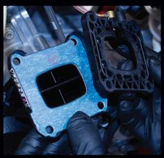
**8)** Prepare new VFORCE4X. Install blue side of gasket with CTR facing you. Install engine side gasket with blue side facing same direction.
