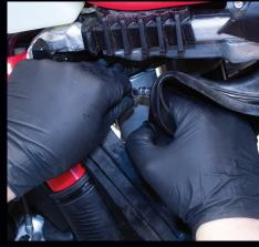
**15)** Reinstall vent hose, then ensure intake boot is fully seated into airbox and "snapped" into place. Tighten airboot hose clamp.
