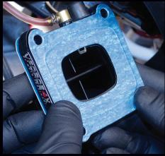
**10)** Put remaining gasket in place lining up bolt holes with blue side facing you.
