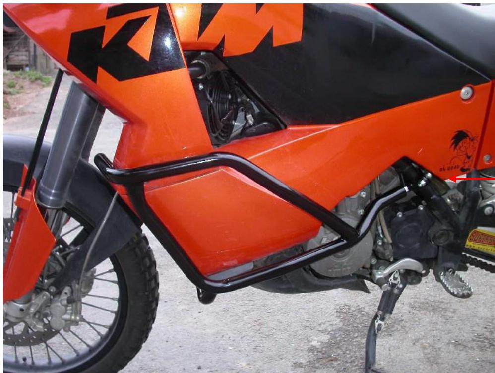
steel adapter with thread M10 + steel adapter on bar  $\varnothing = 25\text{mm}$  + two bolts M8x25mm + four pads M8 (plane) + two nuts M8 (safety)
